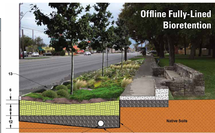
This schematic represents an offline situation where higher flows bypass the system to the existing downstream network. Infiltration is restricted due to hypothetical subsurface conflicts and adjacency to infrastructure.
